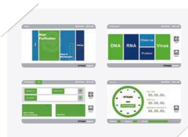
Figure 5. User friendly graphical interface. Integrated computer with 7" TFT LCD touch panel and intuitive OS design. Navigate you to go through purification procedure smoothly.
