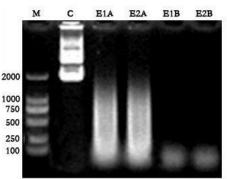
M: Marker; C: Control DNA sample; E1A/E1B: Microccal Nuclease 1U/10U digested DNA(37°C, 5min); E2A/E2B: A commercialized Nuclease 1U/10U digested DNA(37°C, 5min)
